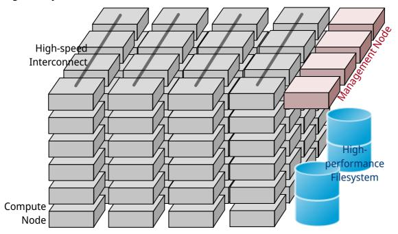
The individual computers/compute nodes are often identical (hardware and software) and are managed by a management node ( management node).
